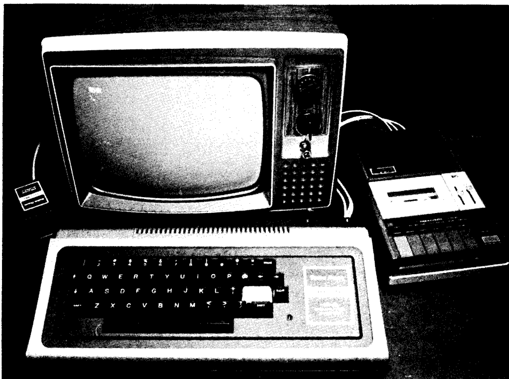
Photo 3: The author's home setup showing the TRS-80 processor unit with its keyboard, connected to an ordinary Hitachi television set modified for direct video entry using a kit from Pickles & Trout, POB 2276, Goleta CA 93018. This setup permits conventional program reception on the television and saves about $100 over the price of the complete Radio Shack system; but it requires some electronics skill in order to modify the television set. Use of this television set and modification kit is further described in the article "Convert Your TV Set to a Video Monitor" which will appear in a forthcoming issue of BYTE.
